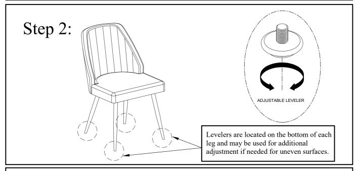
Assembly is now complete and the product is ready for use. Adjustable levelers are located on the bottom of each leg and may be adjusted by turning outwards, counter-clockwise to help account for uneven surfaces. NOTE:Hardware may loosen over time.
