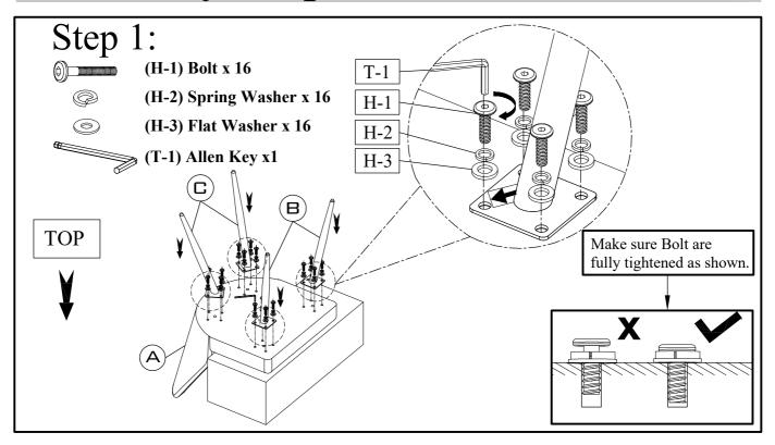
Place Seat (A) upside down on a table top onto a padded, non-marring surface. Position Front Legs (B) and Back Legs (C) onto bottom of Seat (A) so that the directional markings point toward the CENTER of the chair. Secure using Bolts (H-1) Spring Washers (H-2) and Flat Washers (H-3) with Allen Key (T-1), stacking the hardware in the order as shown. Fully tighten all Bolts, but do not over tighten.
